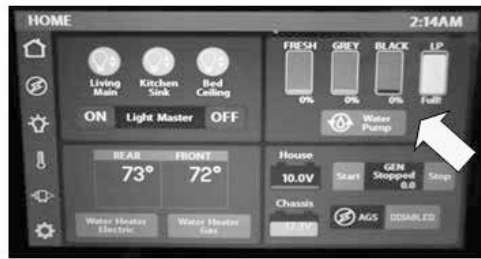
Touch Screen Tank Monitor example
